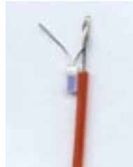
The weld switch (or footswitch) should be pressed and the wires offered to the carbon electrode in the centre of the front panel, the resulting discharge will weld the wires.
