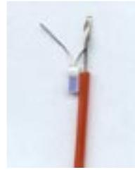
The element wires can be straightened (see fig 4.3b) and insulated as appropriate.
