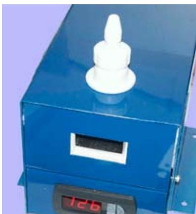
The heater is supplied with 2 PTFE (Teflon) powder-dispensing bottles, one for fine powder and one for coarse. These bottles fit into a hole on the top of the heater where they pick-up heat from the main tube to provide a source of warm dry powder for back-filled Thermocouples and RTD's.
